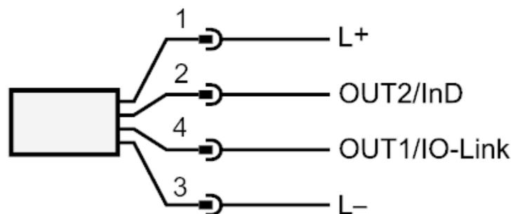
OUT1/IO-Link: switching output volumetric flow quantity monitoring
