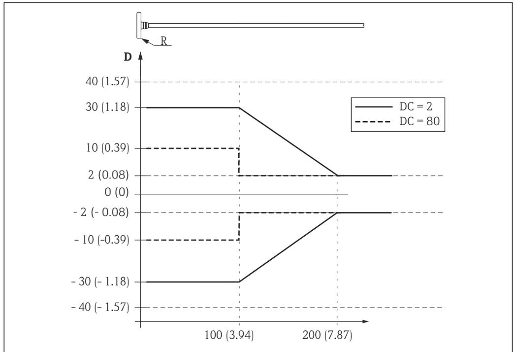
7 Measuring error at the upper end of the probe; dimensions: mm (in)
