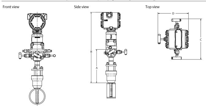
Table 44: 3051CFA Annubar Flow Meter Dimensional Data
