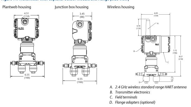
Figure 12: Transmitter with Coplanar Sensor Module and Traditional Flange (Front View)
