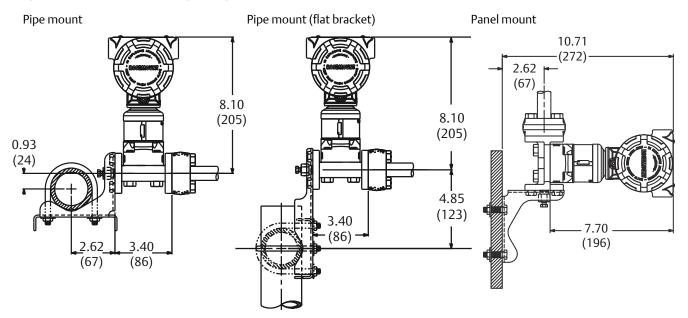
Figure 20: In-line Mounting Configurations (B4 Bracket)
