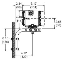
Figure 22: Rosemount 3051SFA Annubar Flow Meter
