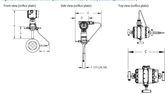
Table 45: Rosemount 3051SFC Compact Orifice Flow Meter Dimensional Data
